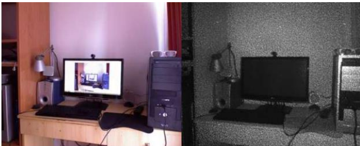
Figure 4 The outputs of the Kinect's colour and infrared camera at a resolution of 1280x1024, even some of the elements of the 9x9 grid can be seen in the infrared picture
